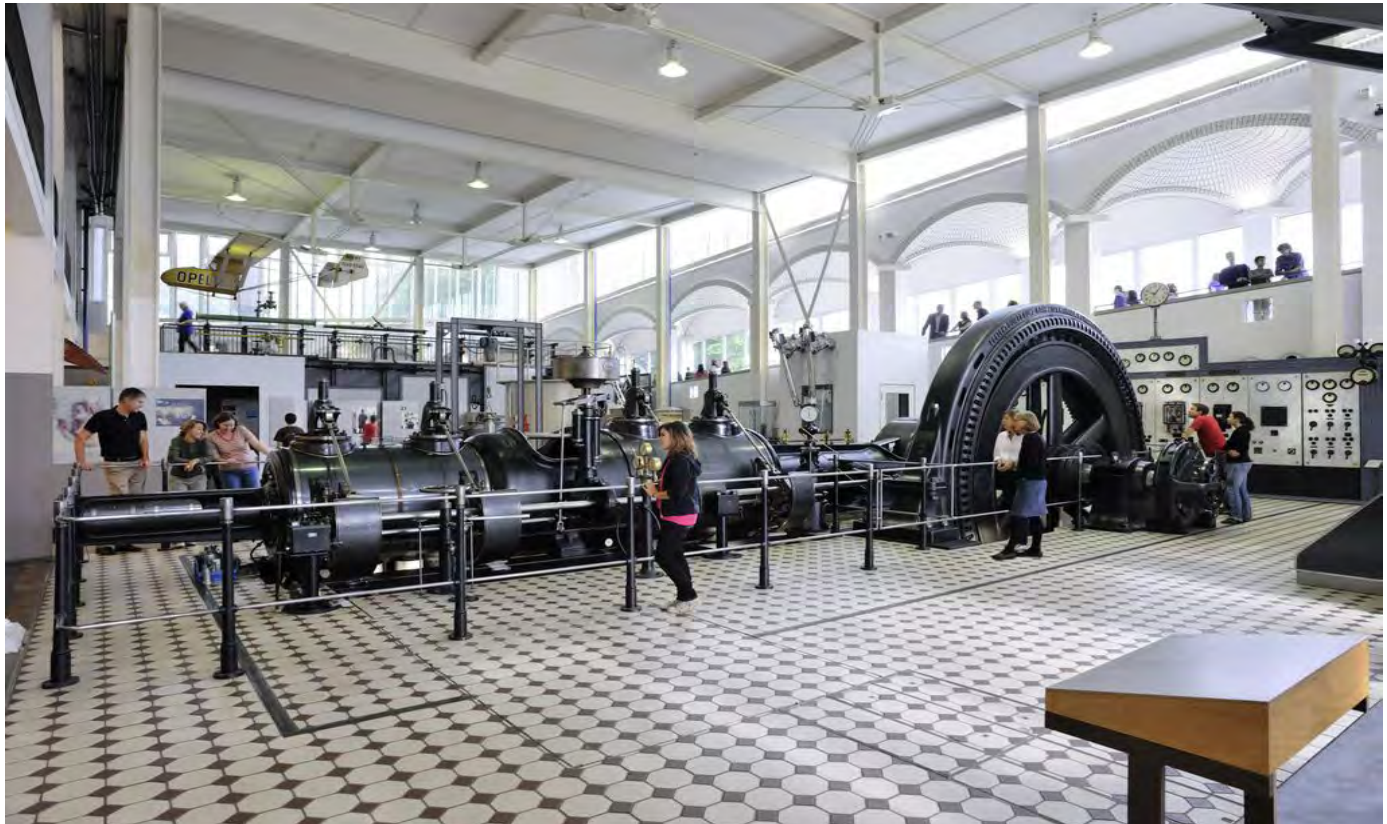
TECHNOSEUM's 500 hp uniflow steam engine built in 1908 by Maschinenfabrik, Esslingen
