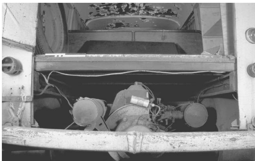
Photo was taken during conservation works. The peeling layers of paintwork at the sealing were stabilised by injecting a solvent-based bonding agent under the flakes, after which they could be reformed using heat and reattached.
