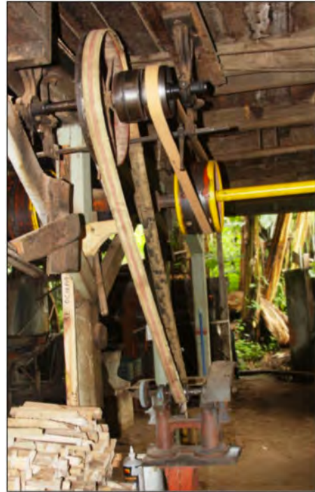
The interior of the cart mill with part of the drive shafting.
