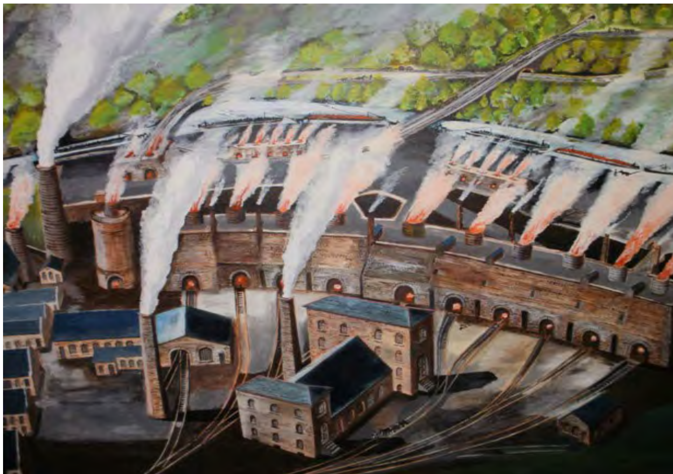
South Wales became the centre of the world's iron-making capacity in the early nineteenth-century with a large group of ironworks. This reconstruction shows the longest single-line of eleven blast-furnaces at Ystalyfera, supplied by the Swansea Canal running along the tops of the furnaces
