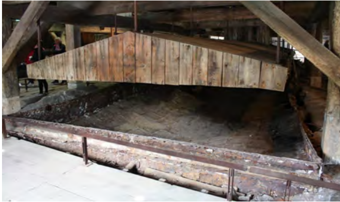
Salins-les-Bains. The last surviving brine sublimation pan, an almost unique survivor in Europe.
