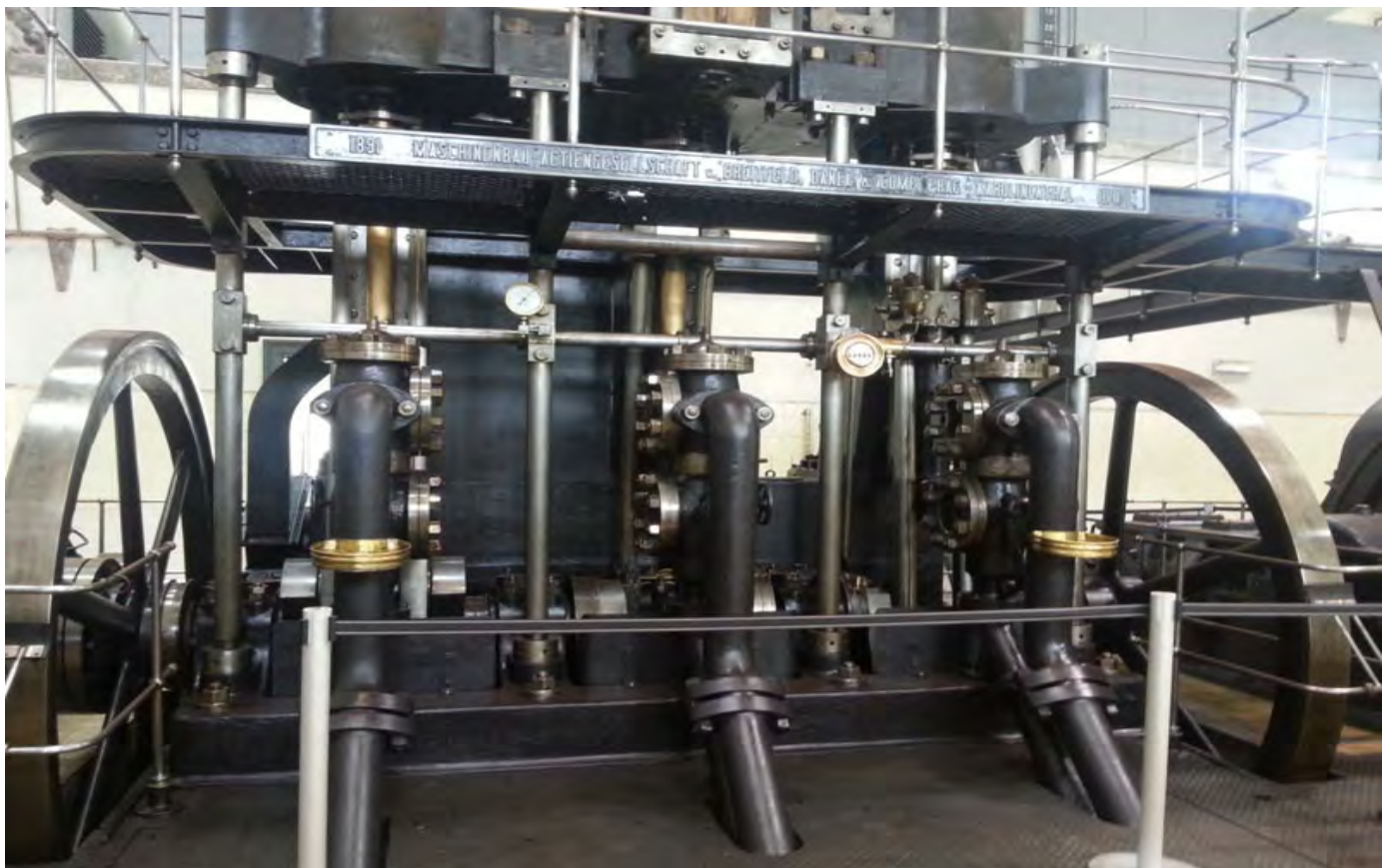
The steam pumping engines were manufactured in 1891 (the fourth one in 1904) in Karlín, today a district of Prague, by Breitfeld - Danek and Company (CKD). Pressure in the hydraulic system could reach 54 bar. Three of them were electrified in the 1930s and one was left intact.
