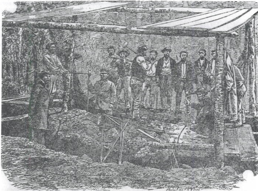
Miners parted large finds of mass copper using sledge hammers and special chisels. (MTU Archives and Copper Country Historical Collections)
