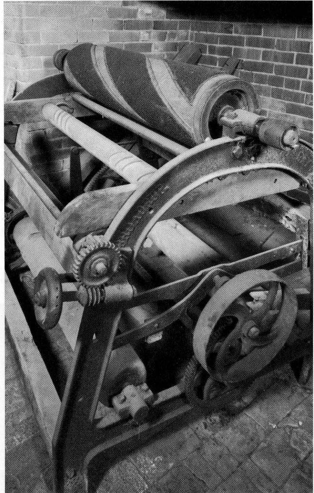
Figure 2. Cloth stretcher manufactured by Broadrup and Co., Dayton, Ohio. Photos by Jet Lowe for Historic American Engineering Record , 1978, unless otherwise noted.
