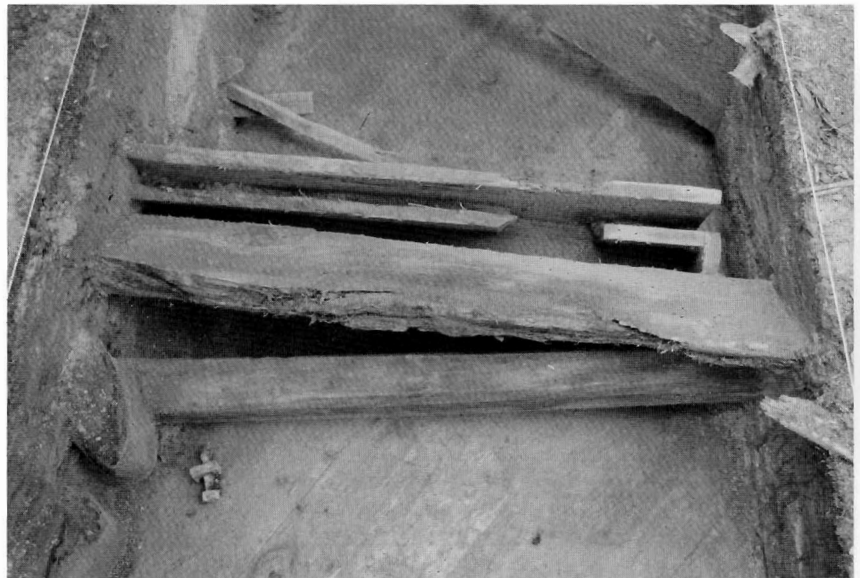
Figure 18. Wooden launder fallen in on the buddle floor. Troughs of this type were used to feed slime onto the center head of the buddle. No good evidence exists to estimate the angle or flow rate at which the launders fed slime onto the buddles.
