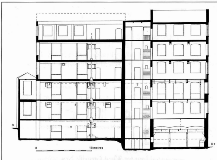
Figure 31 A section through Havelock cotton mill, Manchester, showing the remains of the power transmission system.
