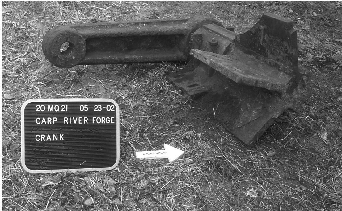
Figure 8. Water wheel gudgeon from the Carp River. The cast-iron flanges on the right would have fit into the end of the water wheel axis timber. The bearing in the center of the gudgeon is held together by four large bolts.
