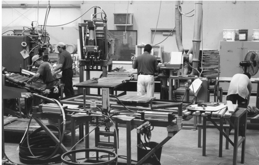
Picture 6: From the right, the heading jointing, heading layout and pinning/squeezing tasks in progress.
