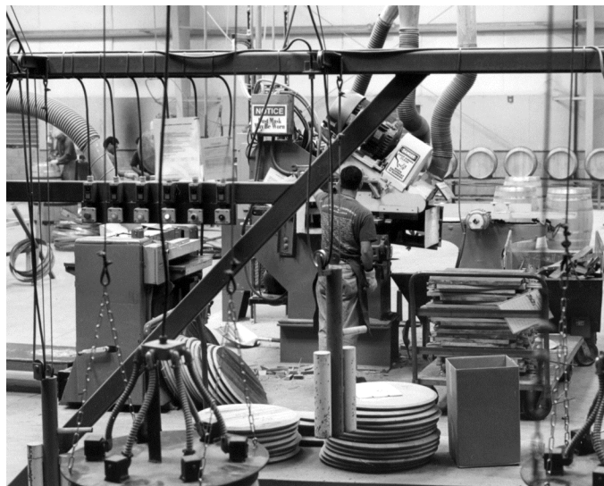
Picture 7: In the background, squares are trimmed into barrel heads. A stack of squares awaits trimming toward the right. Several piles of completed barrel heads are stacked in the center.
