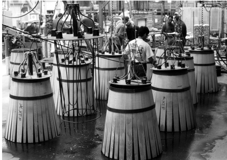
Picture 3: Partially assembled barrels being soaked and warmed in preparation for bending. Note the heater between the two closest barrels.
