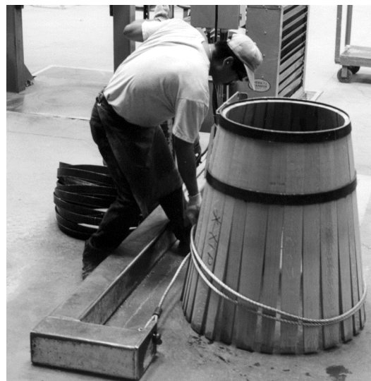
Picture 4: Coiling a steel cable around the bottom of the staves.
