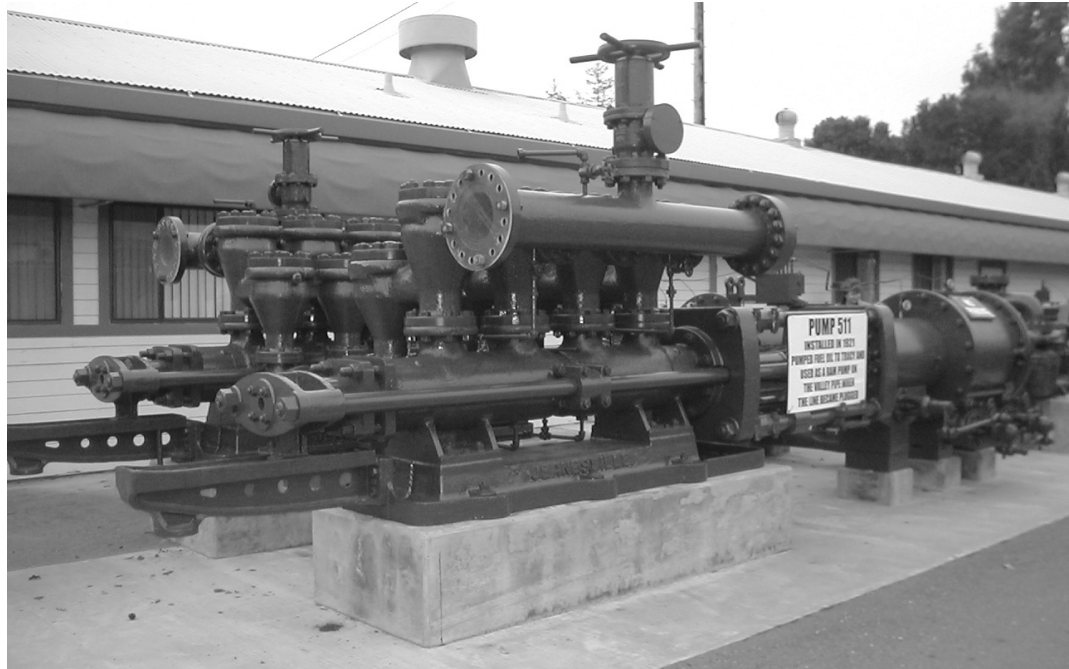
Pump 511. Installed in 1921. Pumped fuel oil to Tracy and used as a ram pump on the Valley Pipe when the line became clogged
