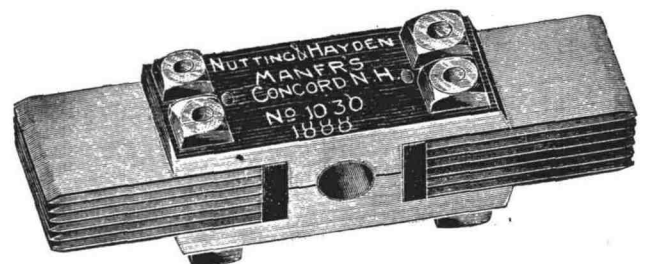
Figure 14. Wood engraving of a bush hammer, from an advertisement for Nutting & Hayden, 1890. The bush hammer, a series of steel plates bolted together and used for dressing stone, was a specialty of Concord tool manufacturers Luther M. Nutting and Henry W. Hayden, in business together from 1888 to 1908. This ingenious tool, with cutting blades that could be readily replaced, was outmoded in the first decades of the 20th century by the pneumatic surfacing machine. A surfacer operator could do the work of 12 men with bush hammers. Courtesy of the New Hampshire Historical Society.
