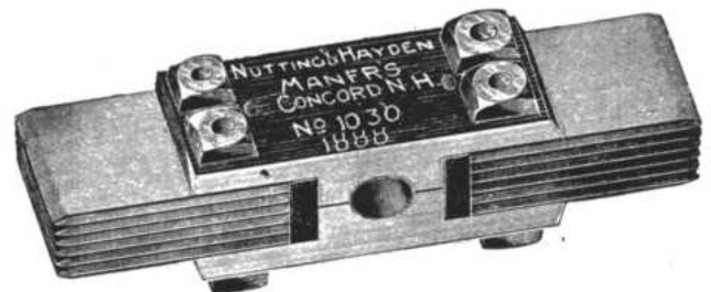
Figure 14. Wood engraving of a bush hammer, from an advertisement for Nutting & Hayden, 1890. The bush hammer, a series of steel plates bolted together and used for dressing stone, was a specialty of Concord tool manufacturers Luther M. Nutting and Henry W. Hayden, in business together from 1888 to 1908. This ingenious tool, with cutting blades that could be readily replaced, was outmoded in the first decades of the 20th century by the pneumatic surfacing machine. A surfer operator could do the work of 12 men with bush hammers. Courtesy of the New Hampshire Historical Society.
