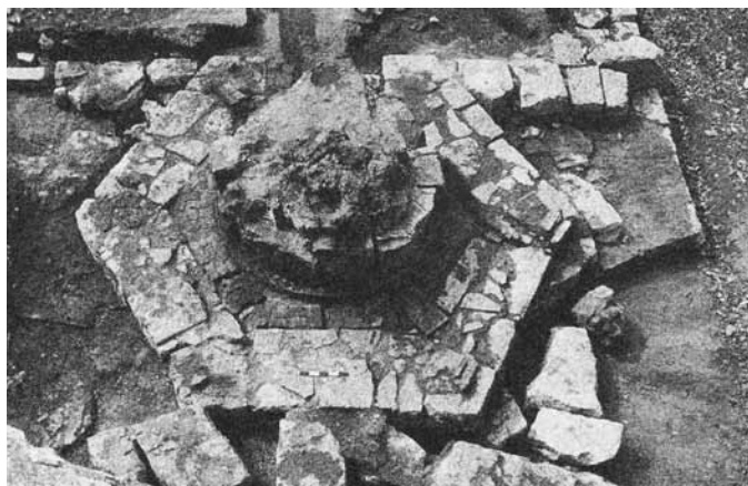
The excavated cupola-furnace base, complete with an iron salamander that marked the furnace's demise in November of 1860. The small scale in the center of the view is 50-cm long.
