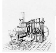
COVER. The illustration on the cover is from A *Treatise* on *the Steam Engine* by John Farey (London, 1827). This ten-horsepower engine, built by Jukes Coulson and Company of London, is remarkably similiar to the engine found in Haiti in 1927. Cornelius Von S. Roosevelt's interesting article on the Haiti engine begins on page 23.
