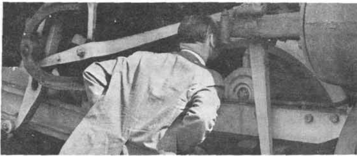
Signs of wear on that front equalizing lever. . . .
