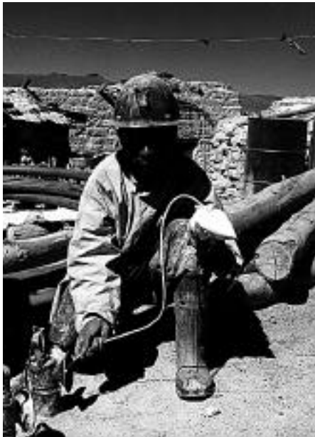
Juan, a former miner and Mark Hufstetler's guide to Cerro Rico, uses one of the carbide lamps to light a length of fuse, which is leading to a plastic bag containing a balled-up stick of dynamite and a bunch of ammonium nitrate. Then boom!
