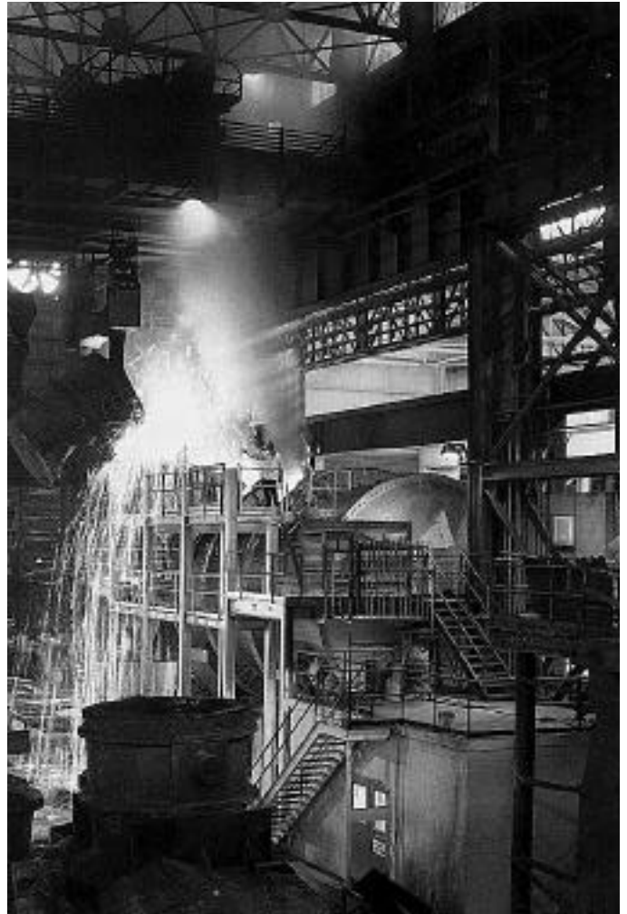
American Cast Iron Pipe Co. After desulfurizing, the iron is conveyed in either a 1300-ton or 1000-ton holding ladle to the centrifugal casters. ACIPCO photo.
