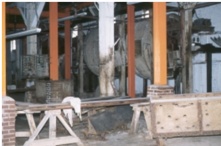
Revolving drums used to pickle sheepskins for shipment to tanneries and skin grading board (1st floor).
