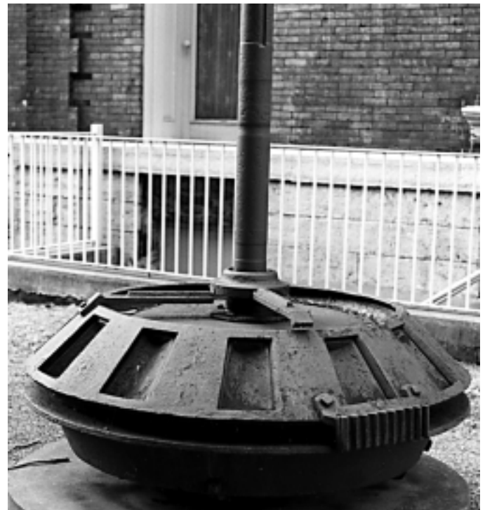
The 36-Inch New American Turbine built by the Dayton Globe Iron Works, Dayton, OH, is one of 34 turbines in the Kinne Collection. This turbine design is based on patents received during the 1850s and 1860s. The turbine operated at the Remington Paper Co., Watertown, NY.
