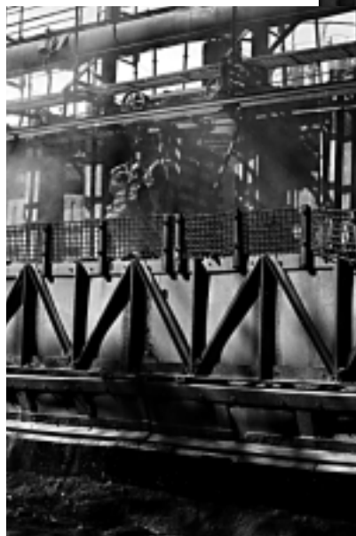
At Empire Coke, a red-hot charge is pushed from a 1913-vintage Semmet-Solvay oven. It then travels by rail to the quenching tower.
