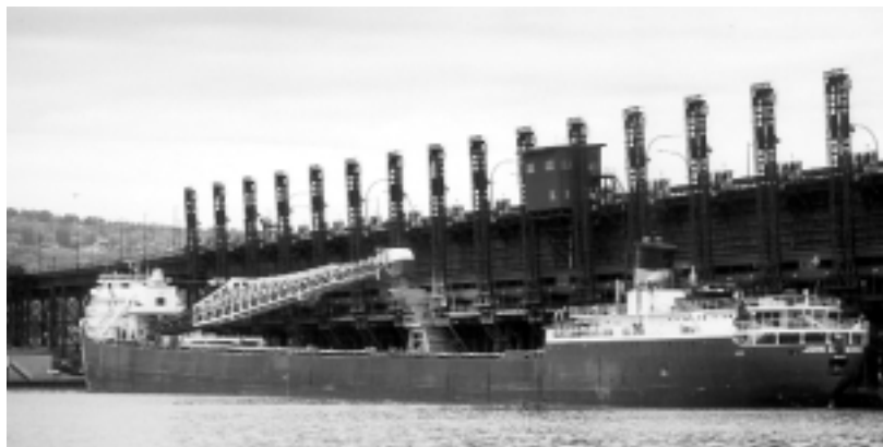
The John G. Munston unloads limestone (to be mixed with taconite for flux at pelletizing plants) before taking on iron at Duluth-Superior Harbor.
