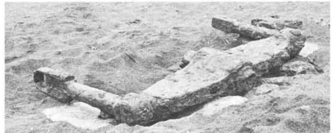
Crosstail of the S.S. Tennessee engine on the beach of Tennessee Cove, Marin Co., Calif. This is the only exposed member of the ship. National Park Service photograph by James P. Delgado.
