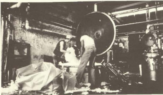
Above: Operating the high pressure, stainless-steel dyeing vats at G.J. Littlewood & Sons, Inc., Dyeworks in Manayunk.
