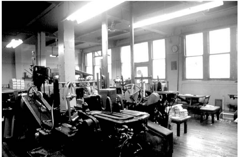
The Stokes & Smith quad-staying machine (ca. 1930-40) at the Chas. M. Jordan Box Co.
