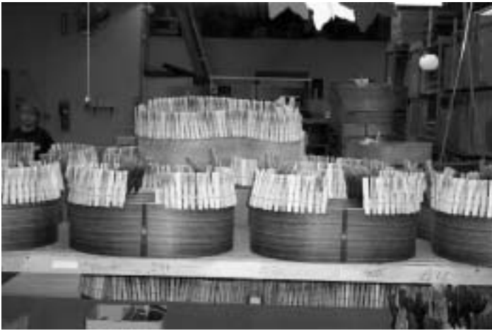
Clamping side pieces to form with clothes pins, Martin & Co.
