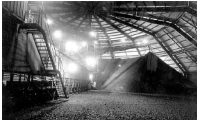
Inside the storage building at Hercules Cement, a system of conveyors continually deliver crushed limestone from the quarry. A slowly rotating radial bulkhead (left) delivers it to secondary crushers and mixers prior to processing in the rotary kilns.
