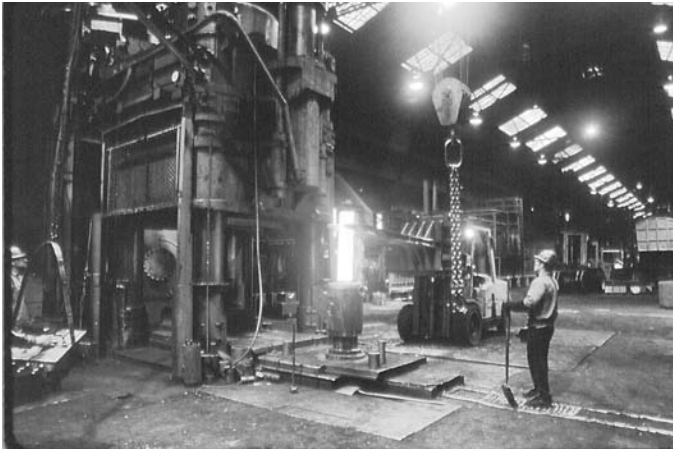
Lenape Forge. A hot blank is about to be lowered into the die (closed-die forging) by a manipulator-equipped forklift, then the table will be rolled back into the press.
