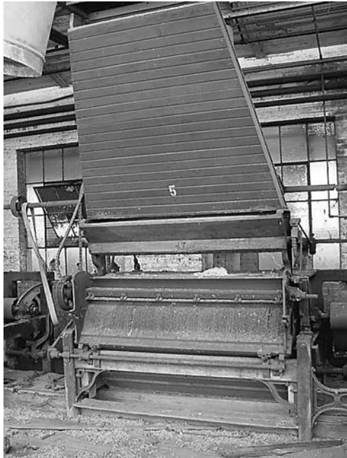
One of the cotton gins still in place in the Union Cotton Oil Mill, 2002.
