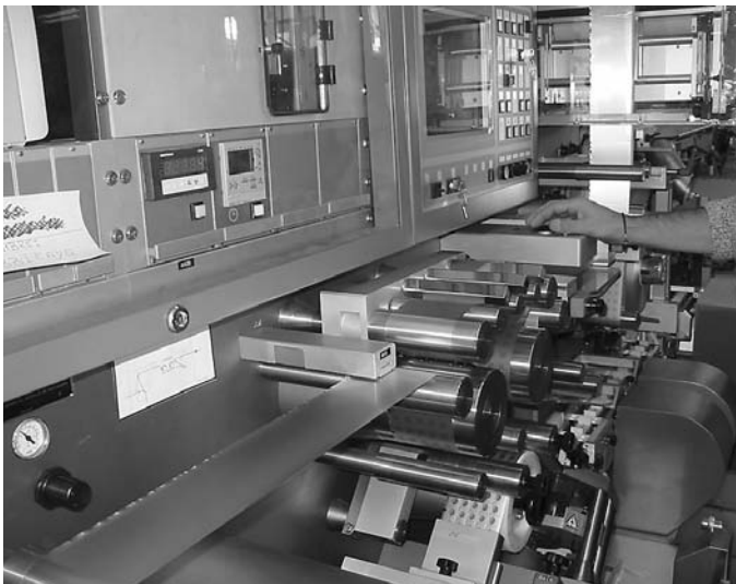
An IMA staff member points out the control panel on the C90 blister pack machine.
