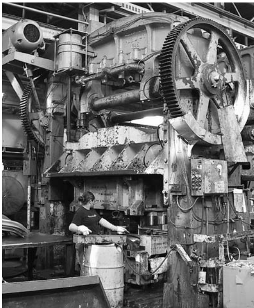
At New Center Stamping, huge presses stamp out replacement automobile parts, including this three-high rack of door panels.
