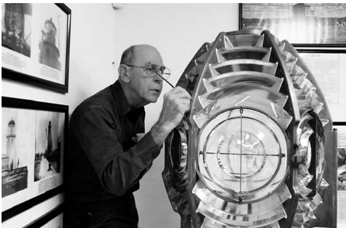
A volunteer cleans the 1896 French-made fourth-order Fresnel lens from the Ashtabula lighthouse, now on display at the Ashtabula Marine Museum.
