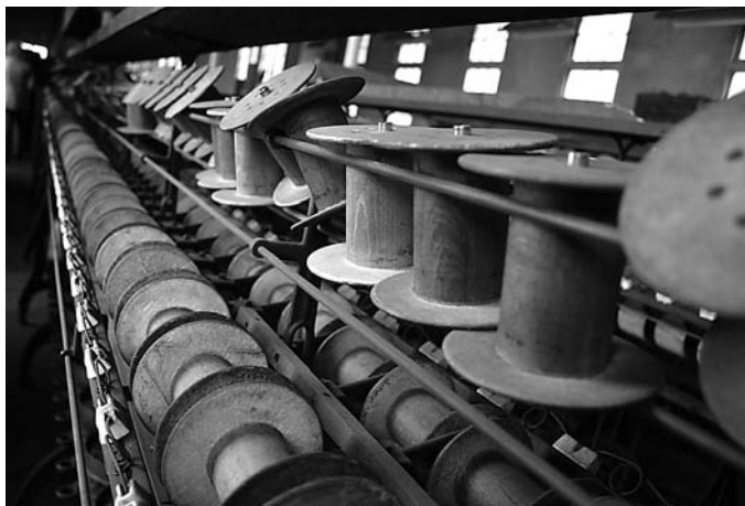
Detail of a spool winding machine, Klots Throwing Mill.
