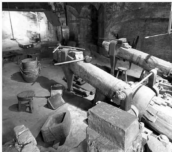
The two tilt hammers and forge at the Farga Ripoll.
