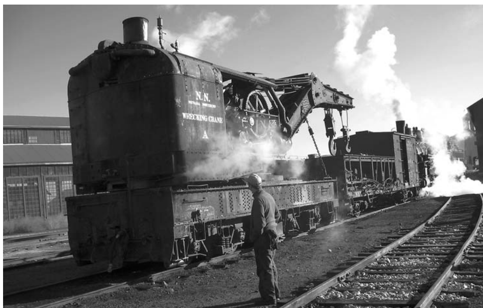
Steaming-up the NNRY wrecking crane.
