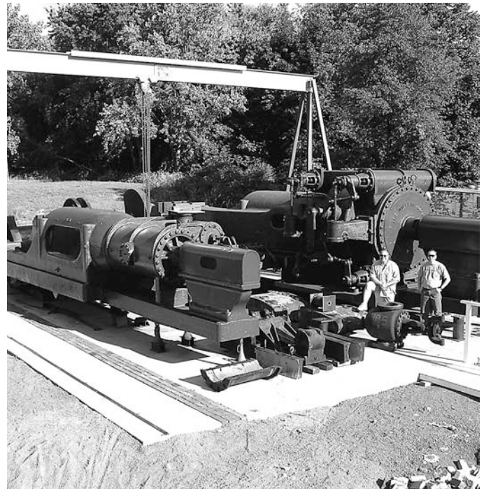
The 1914 Tod Engine. A building will soon surround the massive rolling mill engine that was rescued from the Brier Hill Steel Works in 1995.
