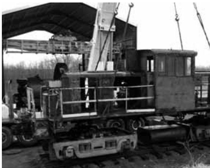
The Youngstown Steel Heritage Foundation's newest acquisition, a 70-ton switcher used in local steel plants.
