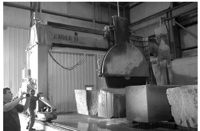
A giant circular saw cuts blocks of granite into slabs at Swenson Granite.
