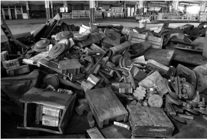
A pile of discarded foundry patterns at the former Beloit factory.
