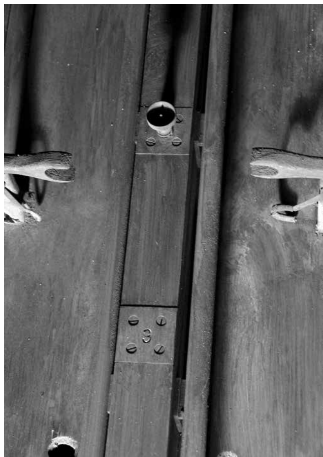
Top of Type X instrument box, showing plate with number "3", small cupped knob, tubes, and hooks/seats for glass tubes (not shown).
