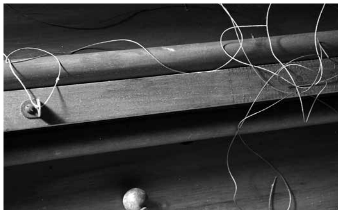
Top of Type Y instrument box showing string and spherical end weight, and steel tube at top.
