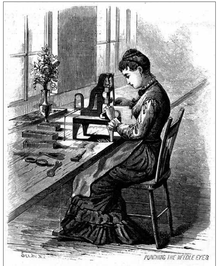
Punching the needle eyes at Wheeler & Wilson Manufacturing around 1889.
