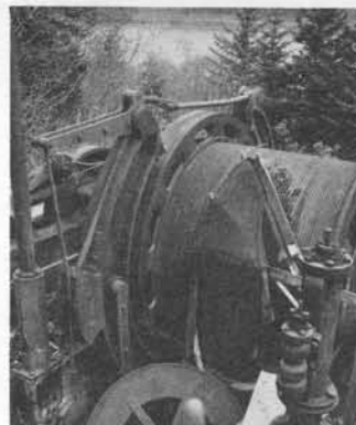
The partially dismantled remains of an Allis-Chalmers steam mine hoist from the Treadwell group of mines, Douglas Island.
