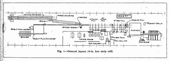
The fling shear is an Edwards steam operated type; the width of the knives is 10 in. and the diameter of the steam cylinder is 12 in.
